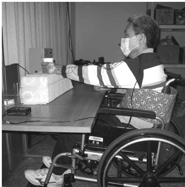
Figure 1. Experimental setup for stroke subjects to perform a reaching movement.
